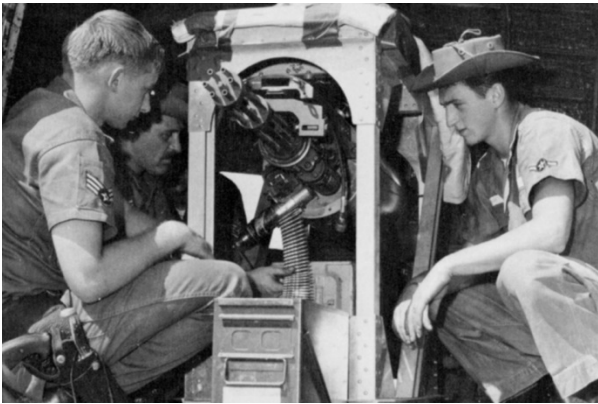
One of the fabricated mounts for the SUU-11/A minigun pods aboard the original "Puff the Magic Dragon" C-47 gunship. (U.S. Air Force)
