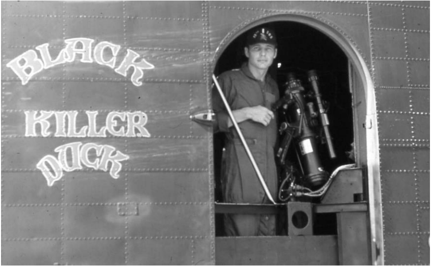
Lt. Barbee at the Night Observation Sight (NOS) position. Courtesy of Frank Baehre.
