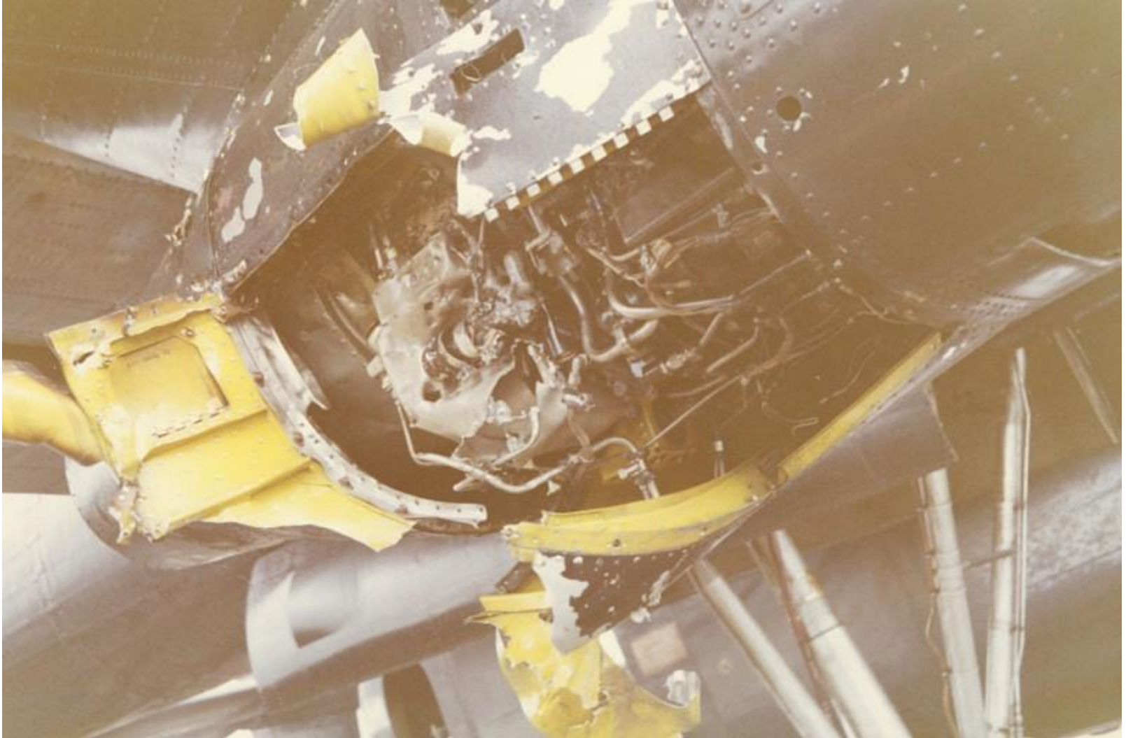
AC-119K J85 JET ENGINE WITH BATTLE DAMAGE
